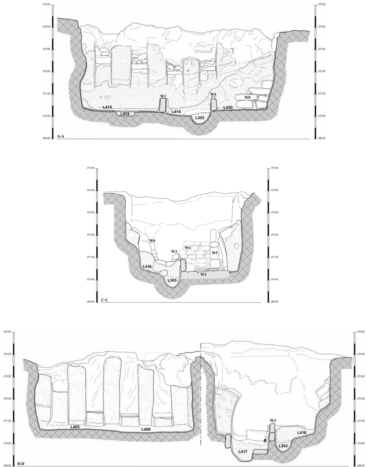
Fig. 10.2. Sections of the two Arched Reservoirs.
